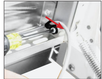
FIG. 7. Pull the reed switch wire through the rainshield bushing.
