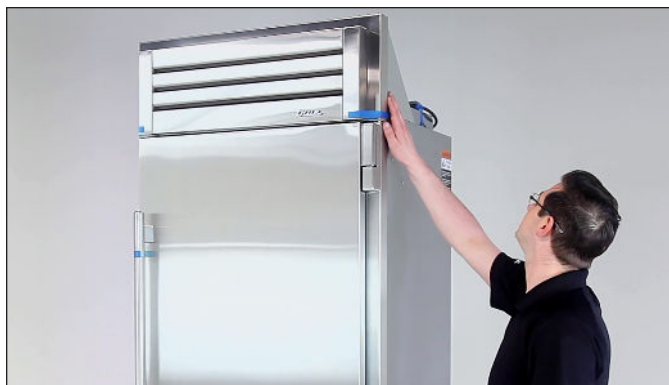
FIG. 2. Inspect the unit's exterior for visible damage.
