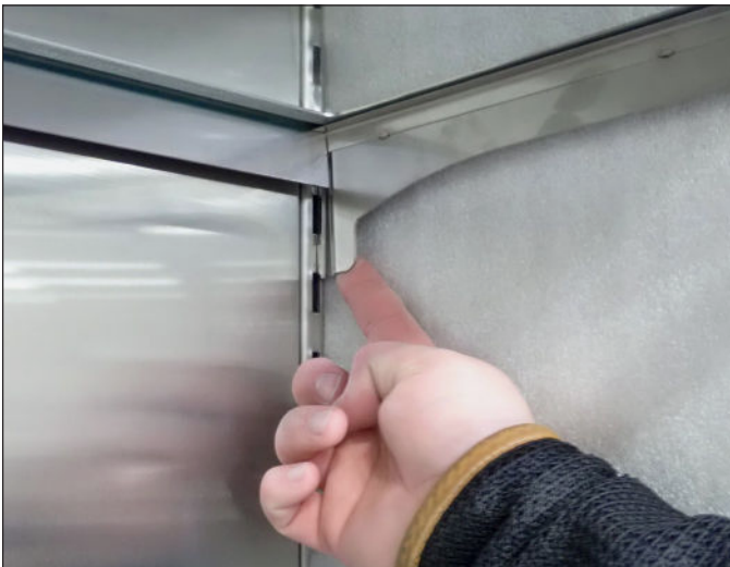
FIG. 6. Push the bottom tab inward.
