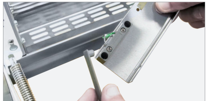
FIG. 4. Remove the plastic cover.
