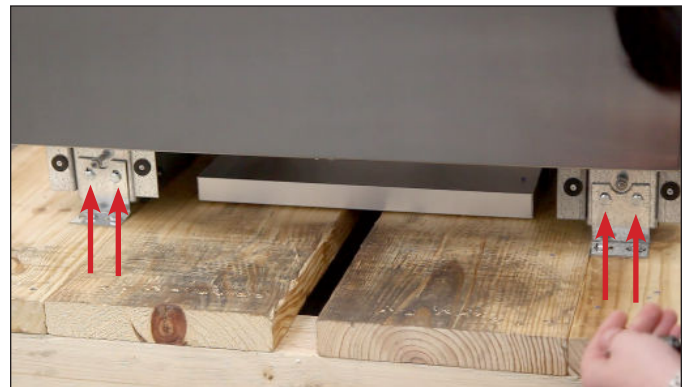
FIG. 7. Shipping bracket bolt locations.
