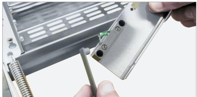
FIG. 4. Remove the plastic cover.
