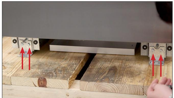
FIG. 7. Shipping bracket bolt locations.
