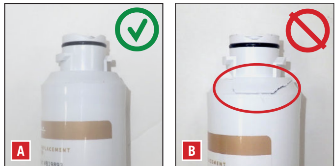
FIG. 4. Undamaged water filter head (A) vs. a damaged water filter head (B).
