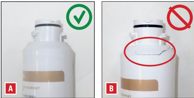
FIG. 5. Undamaged water filter head (A) vs. a damaged water filter head (B).
