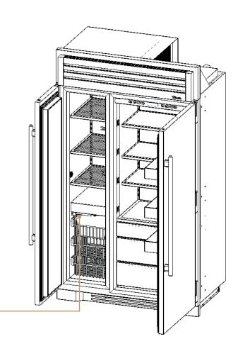
Serial label located on the interior left wall of the freezer when the top wire basket is pulled out
