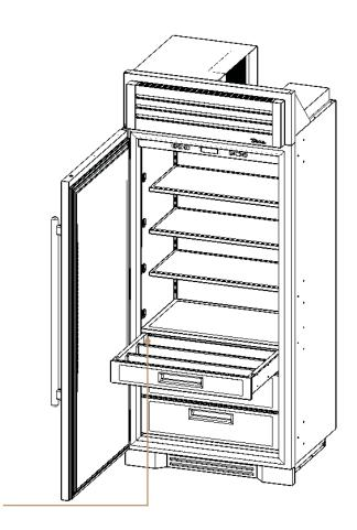
Serial label located on the interior left wall when top drawer is pulled out -
