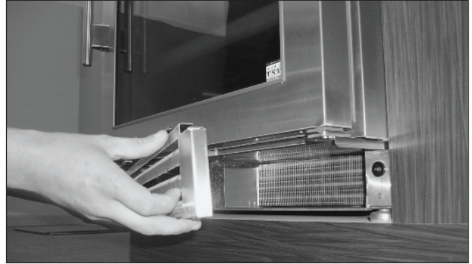
FIG. 1. Carefully remove the kickplate.
